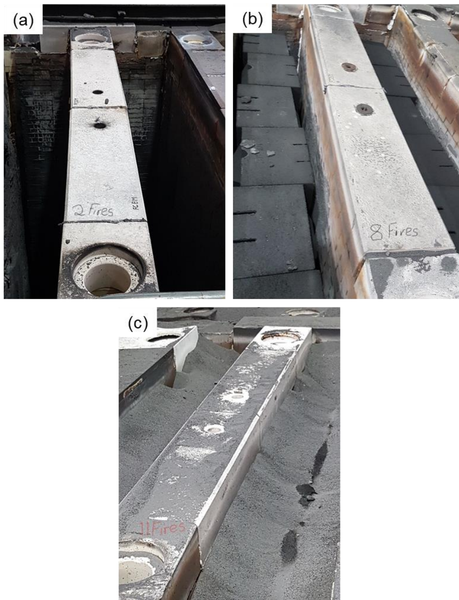
Figure 7 - ThermStop Concept™ top blocks with distinct fire cycles: (a) 2 fires, (b) 8 fires and (c) 11 fires.
