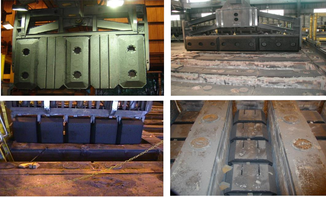
Figure 3 - Loading / unloading anodes can cause mechanical damages.
