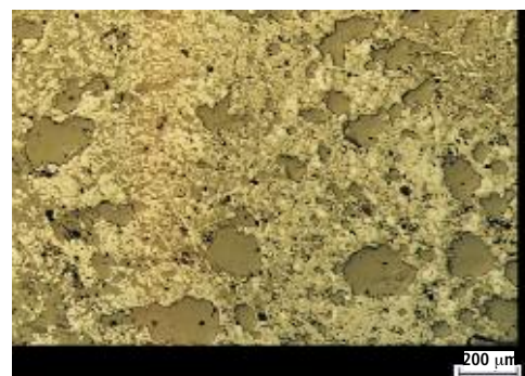
Fig. 3 Texture after the corrosion test
